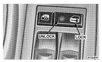
Vehicles equipped with power door locks can be locked or unlocked from inside by either the use of the door lock switches located on the front doors or by pressing the LOCK or UNLOCK buttons on the Remote Keyless Entry key fob.
